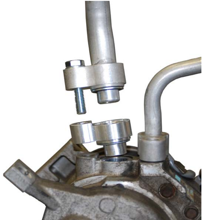
T95-1453 Denso 10S17F Plate Installation
